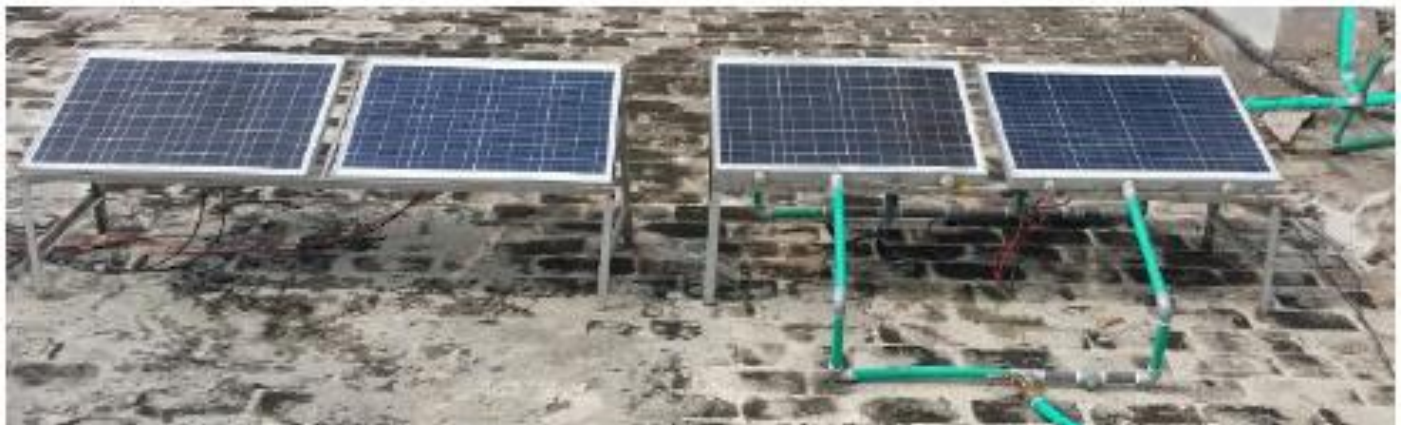
Figure 4: Experimental set-up; PV modules with cooling and without cooling
